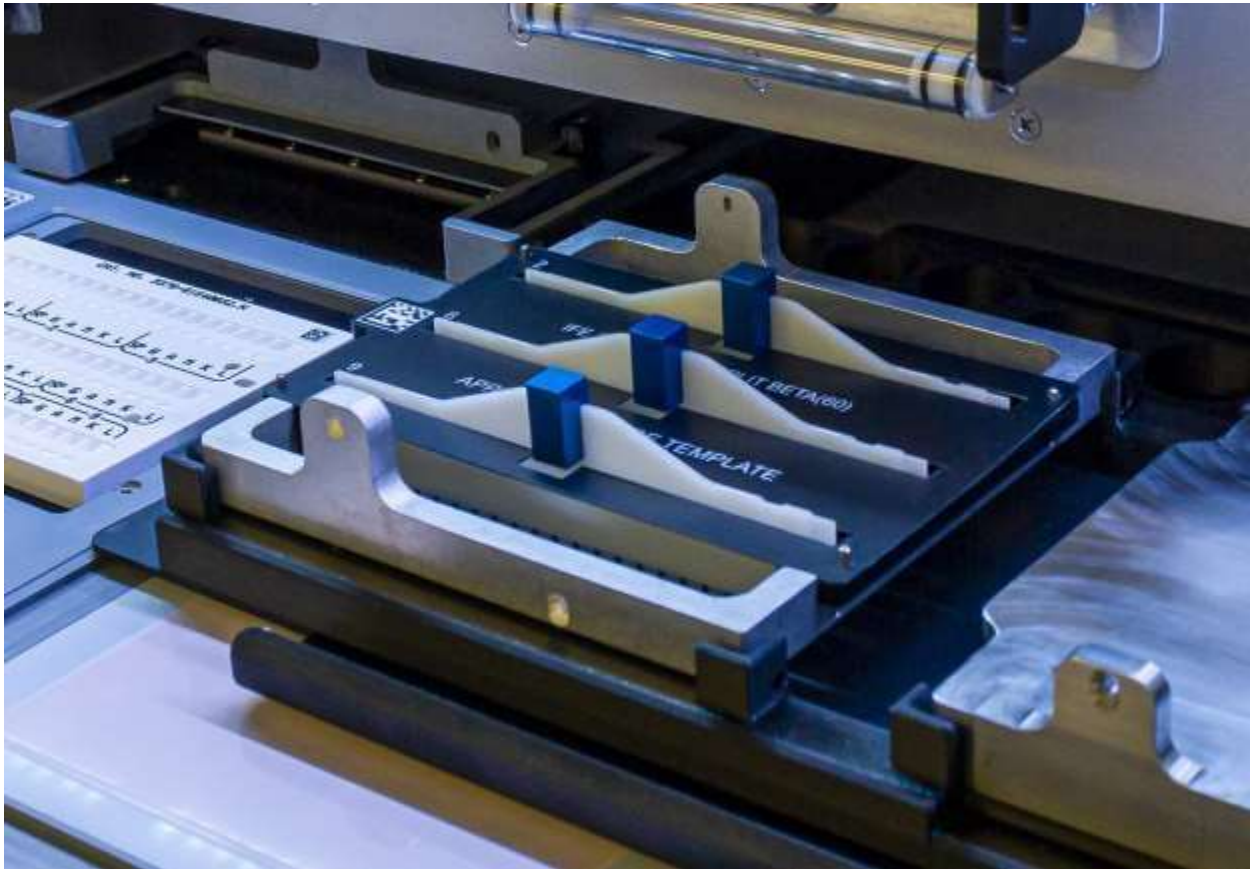
Figure 7-15 Applicator Holder with Applicator Blades, Applicator Blade Template, and Blade Weights
